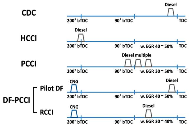
Figure 4. The fuel supply concepts of CI and various advanced combustion technologies
