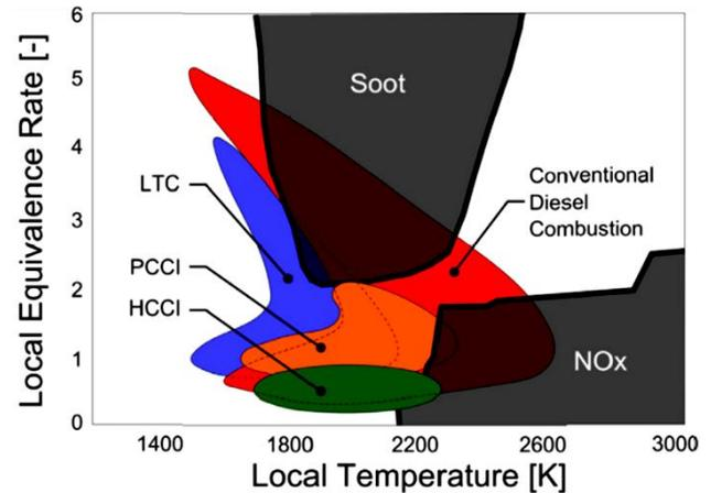
Figure 3.  $\Phi$ -T diagram of different combustion modes: CI, HCCI, and PCCI, on soot-NO<sub>x</sub> map
