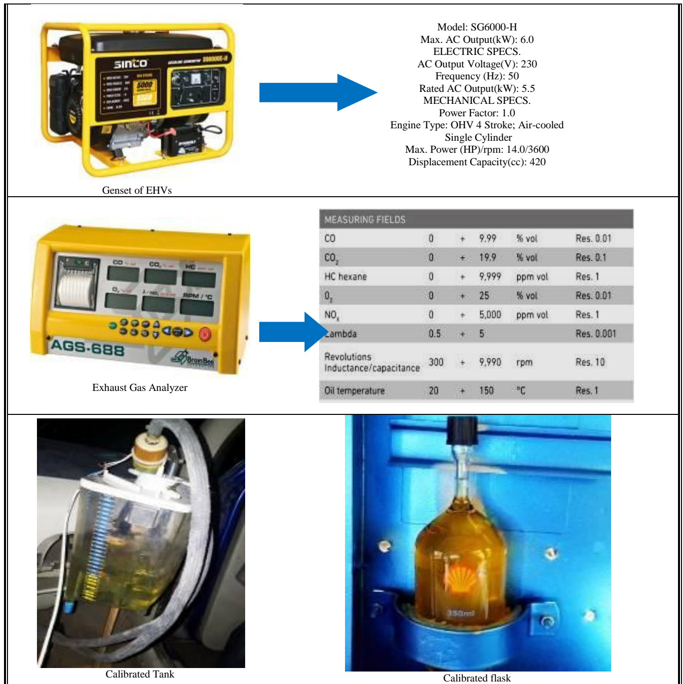
Fig. 9: System qualifications, measurement variety, and error of engines, gas analyzer, and calibrated tank and flask
