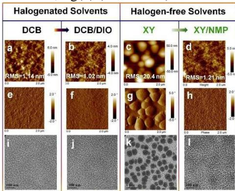
**Figure (3):** AFM topography (a, b, c, d), phase (e, f, g, h) and TEM (i, j, k, l) images of the films cast from: DCB, DCB/3% DIO halogenated solvents, XY and XY/2% NMP halogen-free solvents, respectively
