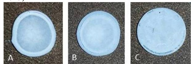
**Figure (4):** Coffee ring effect observed in deposited drops for different concentrations by weight of PEG20000 relative to TiO<sub>2</sub>: A) 10%, B) 20%, and C) 50%
