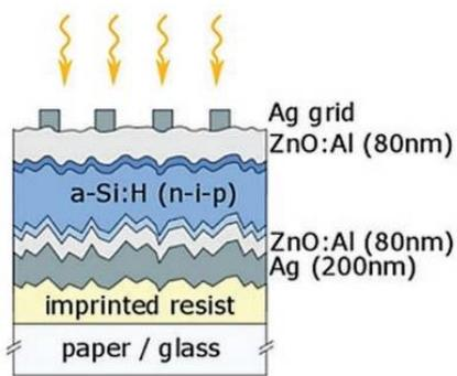
**Figure (2):** paper surface modification with a UV resistive resin. Resin allowed a controllable design of surface pattern that enhanced the light scattering in an a-Si solar cell (Smeets 2017)5.3: Challenges in using Inkjet Printing
