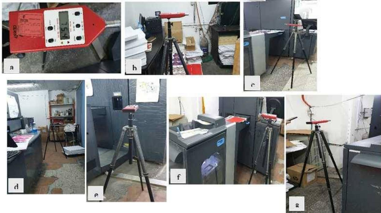
**Figure (2):** The experiment on site (room 1) while measuring sound levels: a) QUEST noise level instrument, b) Point 1 measurement, c) Point 2 measurement, d) Point 3 measurement, e) Point 4 measurement, f) Point 5 measurement, g) Point 6 measurement
