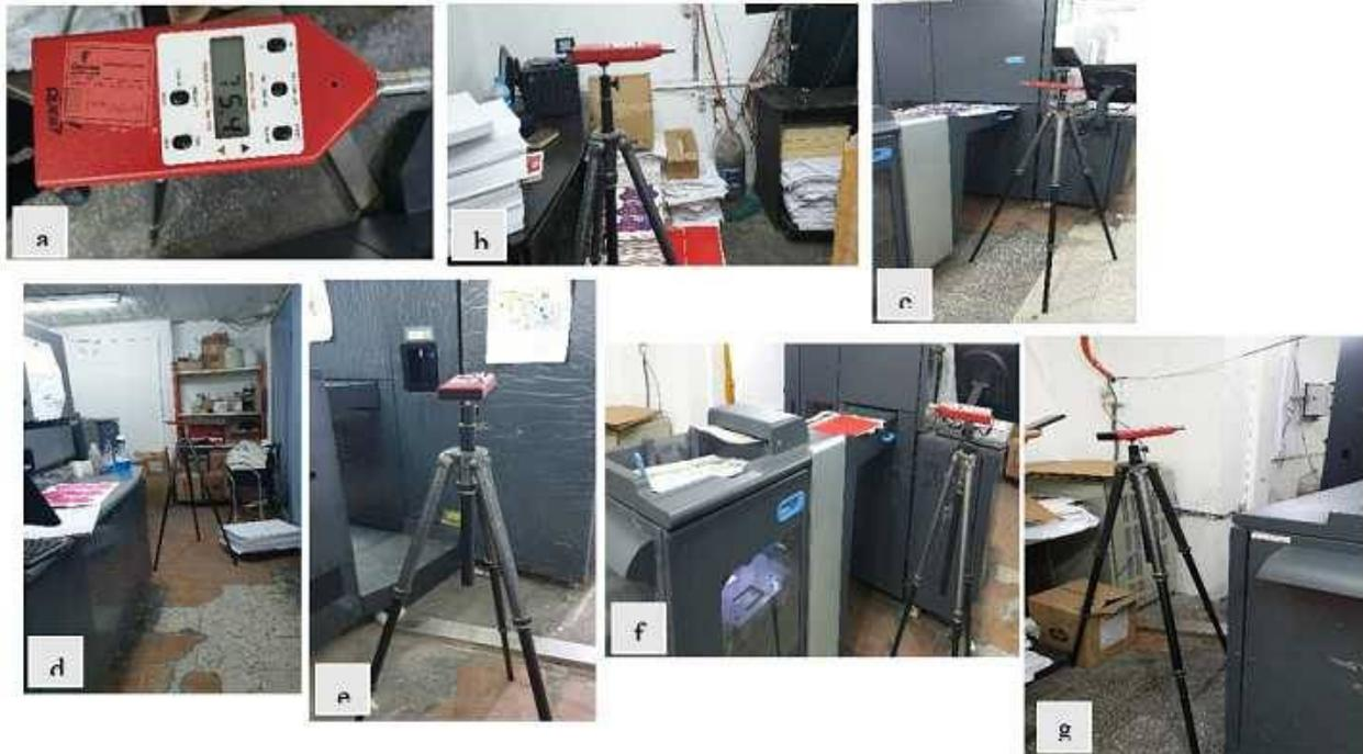
**Figure (3):** The experiment on site (room 2) while measuring sound levels: a) Two Xerox WorkCentre 5875 Digital printing presses , b) HP Indigo 7800 Digital Press Chiller , c) both of machines set – up places
