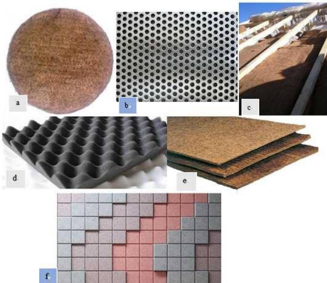
**Figure (4):** Suggested eco- friendly acoustic sound absorber panel includes: a) Jute material panel. b) Micro Perforated Pates (MPP) which can be integrated with jute material to increase jute panel sound absorbing performance. c) Thermal jute. d) Eco Plastic foams panel. e) Coconut fibre sound absorber panels. f) Baux sound absorb Wood Wool resistant fire eco-friendly 3D panel model
