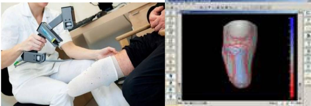
**Figure (9). 3D surfaces by gathering measurements made by smoothly sweeping a handheld laser scanning wand**
