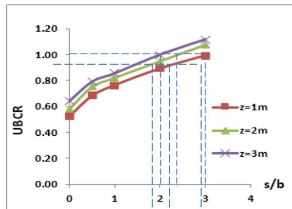
Fig. 12: Variation of UBCR with spacing between footings ( $s/b$ ) resting over different thicknesses ( $z$ ) of a sand cushion replacement.
