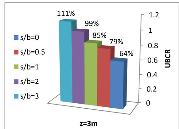
Fig. 16: The percentage increase of the UBCR for different spacing ratio (s/b) in case of a replaced sand cushion of (z = 3m).
