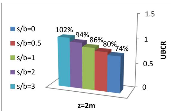
Fig. 18: The percentage increase of the UBCR for different spacing ratio (s/b) in case of a replaced reinforced sand cushion of (z = 2m).
