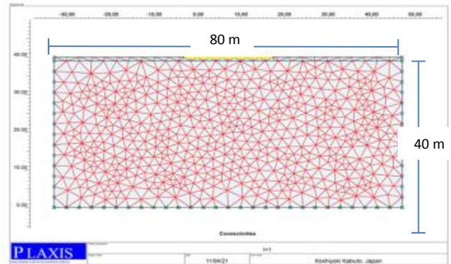
Fig. 2: The mesh of FE modeling of two strip footings on semi-infinite homogenous clay soil.
