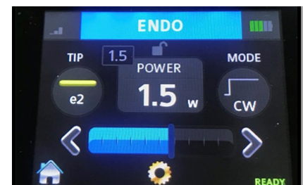
Figure 5. Diode laser (Epic X™, BIOLASE, USA) with an output power 1.5 Watt
