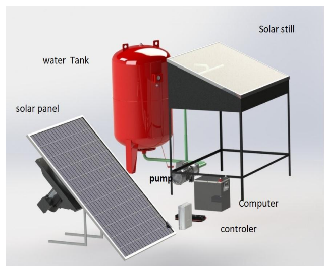
Fig. 2: Schematic diagram for the experimental setup
