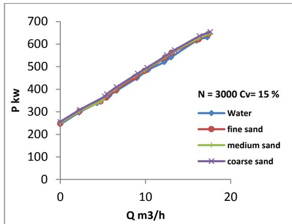
(b) Power-Capacity Characteristics
