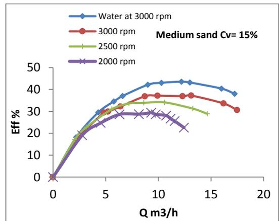
(c) Efficiency-Capacity Characteristics
