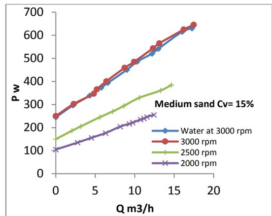
(b) Power-Capacity Characteristics
