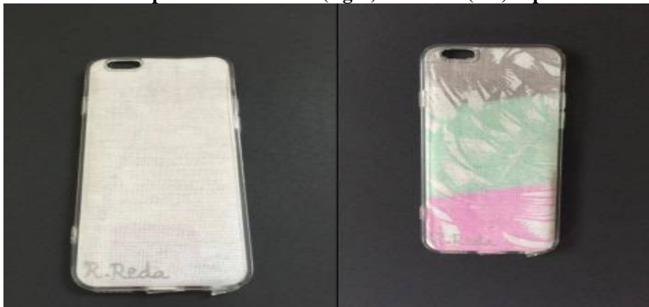
Figure 4.6 the smart phone cover before (right) and after (left) exposure to the heat
