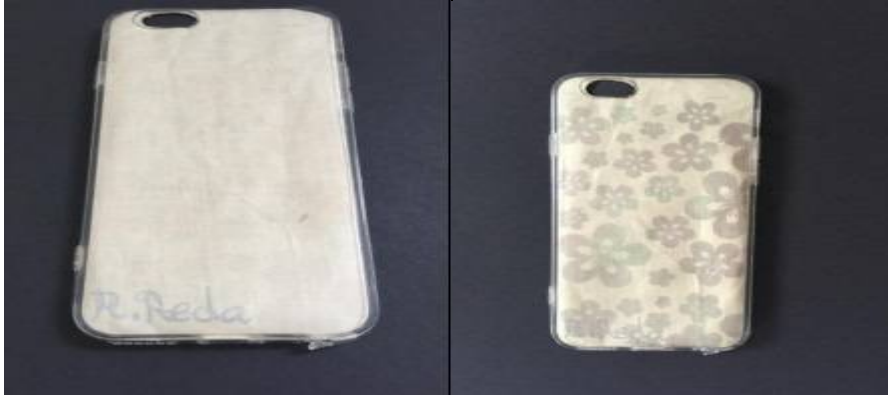
Figure 4.5 the smart phone cover before (right) and after (left) exposure to the heat
