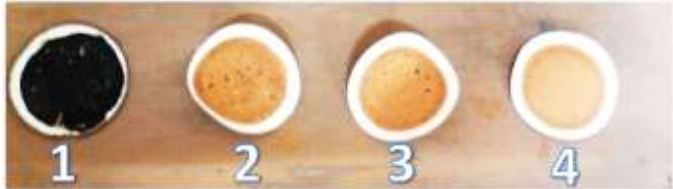
Fig.5: shows decreasing in organics in substrate after each fermentation cycle: 1)after first dark cycle, 2) after first photo cycle, 3)after second dark cycle and 4)after second photo cycle.
