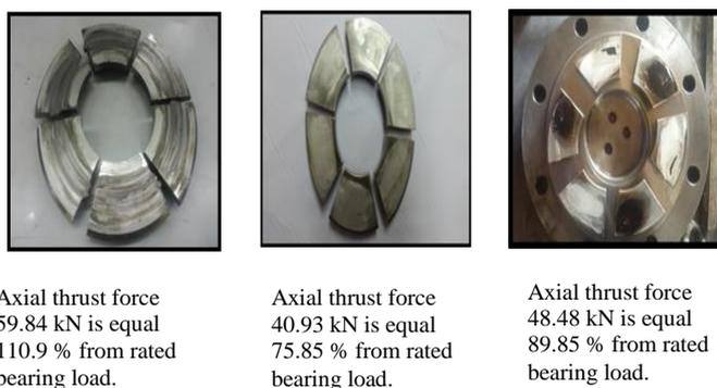
Fig. 13: Axial Thrust Force Effect on Thrust Bearing
