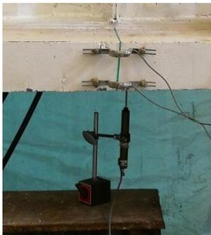
Fig. (11) Positions of LVDT under the applied load ( $\delta_1$ ) for all specimens
