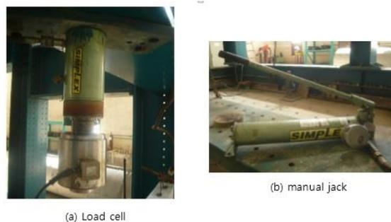
Fig. (14) Load cell and manual jack
