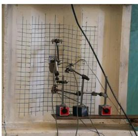
Fig. (12) Positions of LVDTs used to measure the out-of-plane displacement ( $\delta_01$ ), ( $\delta_02$ ) and ( $\delta_03$ )
