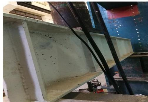
Photos of specimen G7-350-S (Steel only) after failure
