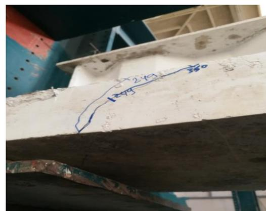
Photos of specimen G8-350-T (no fiber) after failure
