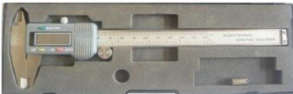
Fig.(17) digital side calipers
