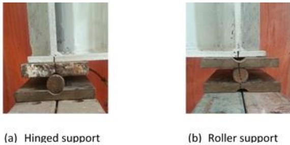
Fig. (10) End conditions used in the tests
