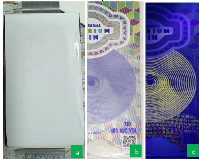
Figure (14): a) Design 2 Group A wetted test result (blank paper) after 25 stroke sequence, b) design 2 Group A sample visible ink after wetted rub test, c) design 2 Group A sample invisible ink after wetted rub test
