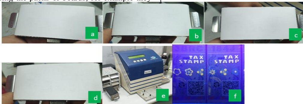
Figure (8): a) Test result after 25 stroke sequence, b) Test result after 75 stroke sequence, c) Test result after 100 stroke sequence, d) Test result after 150 stroke sequence, e) Ink rub tester, f) Design 1 under UV light source after end of dry ink rub test
