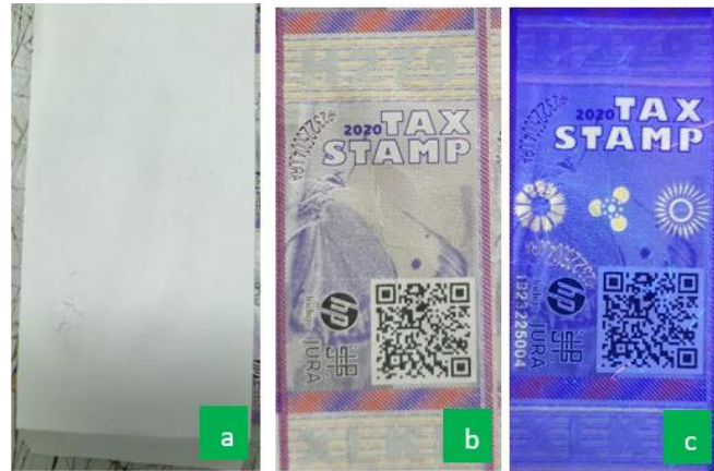
Figure (13): a) blank paper fibres damaged after 3 wetted stroke sequence, b) design 1 sample visible ink after wetted rub test, c) design 1 sample invisible ink after wetted rub test
