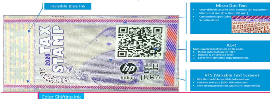
Figure (2): Tax Stamp design security elements/ designed by JURA Corvina Security Designer Program
