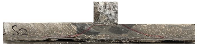
(b) Crack patterns of S2
