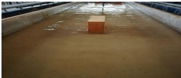
Figure 2. A modeled rectangular bridge pier at the considered laboratory flume.
