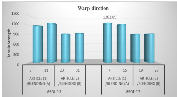
Fig. (12&13) shown the relation between Group (3&7) to found the effect of shedding angle on specimen's tensile strength at 3kn warp tension with 46 pick / Inch for both directions.
