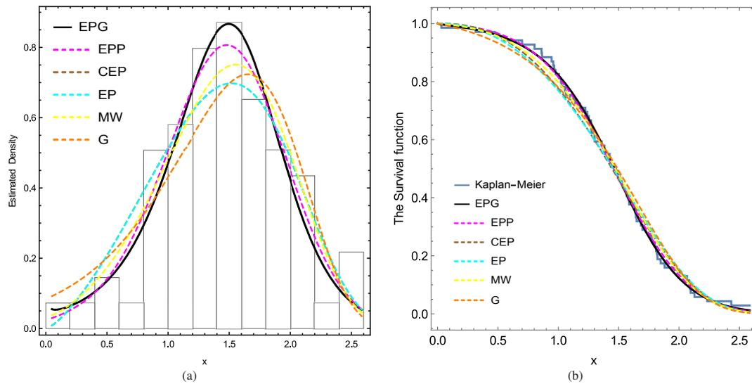
Fig. 3: Turbocharger dataset: (a) empirical and fitted densities (b) Kaplan-Meier and fitted survival curves
