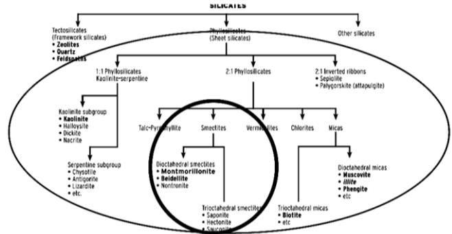
Figure 2. Classification of silicates and bentonite [18].
