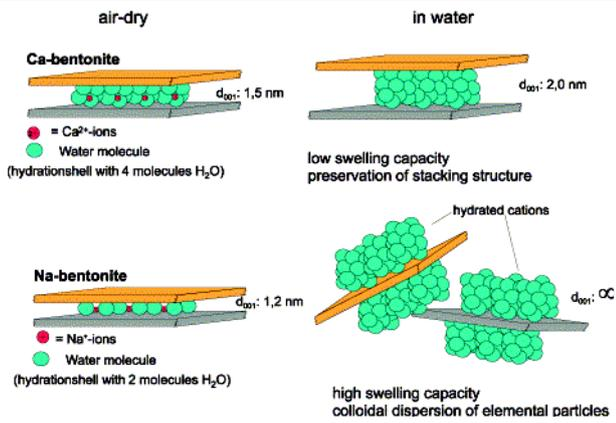
Figure 1. Intracrystalline swelling of calcium and sodium bentonite [17].
