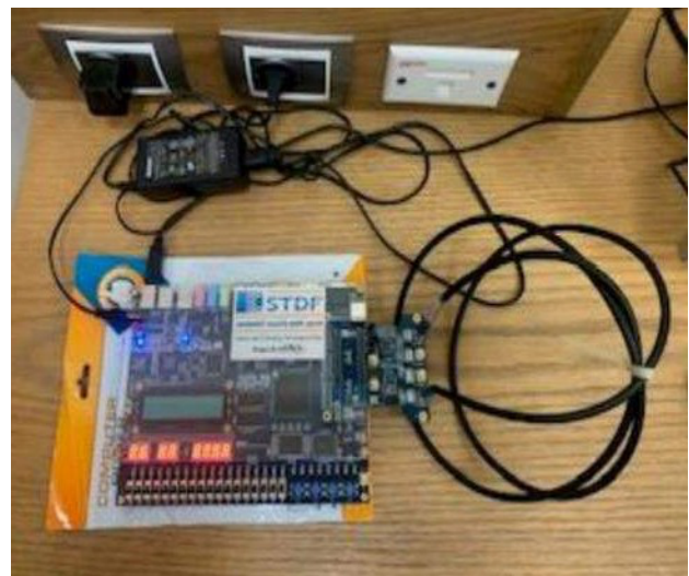
Figure 7: Experimental setup for the Altera DE2-70 board, with the A/D converter card
