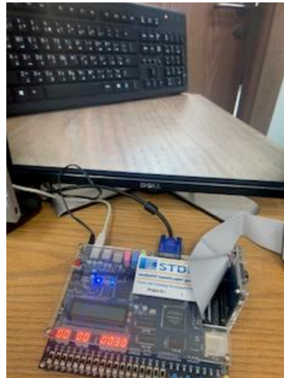
Figure 6: The DE2 board, with the VGA monitor, and the D5M Camera (Camera initialized)
