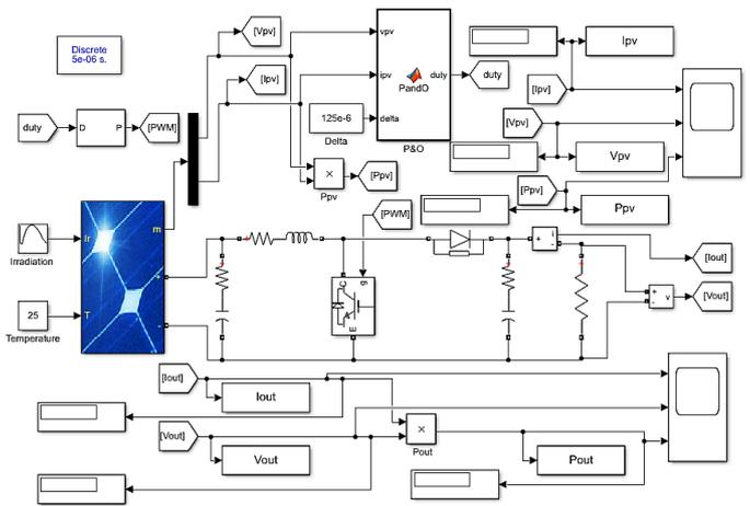
Figure 7. The block diagram of P&O MPPT controller.
