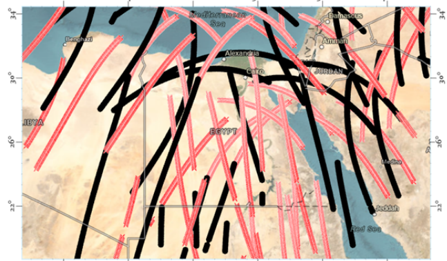
Figure (5): IPP tracks over Egypt for GPS and GLONASS satellites observed at 0-2 am on May 10, 2015, at ALAM, ASWN, MTRH, and SAID.
