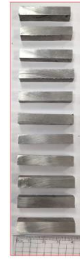
Figure 4. The samples before undergoing ECAP, with Teflon used to secure them in a bent configuration.
