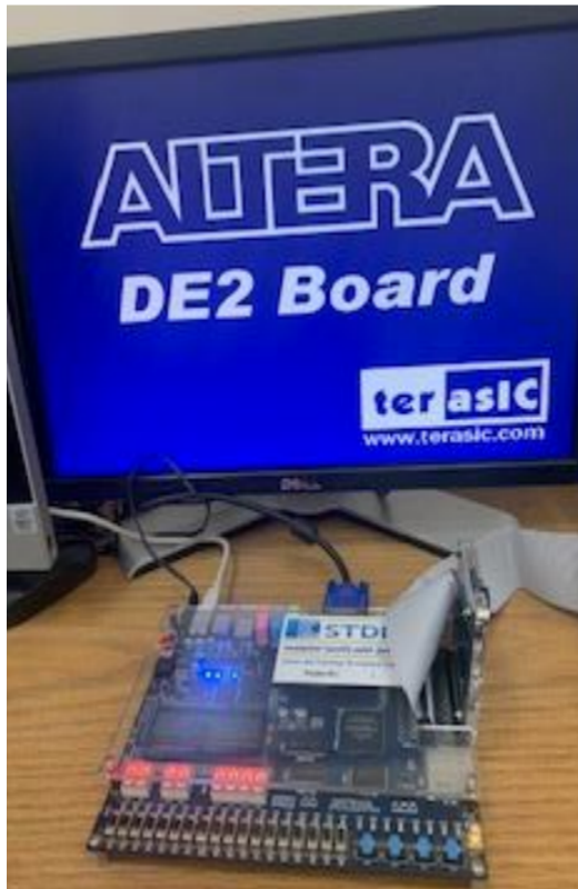
Figure 5: The DE2 board, with the VGA monitor, and the D5M Camera (Camera not initialized)
