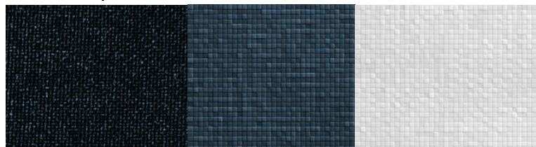
Figure (1) Plain 1/1 weaving structure Sample Code: 5 1 8
