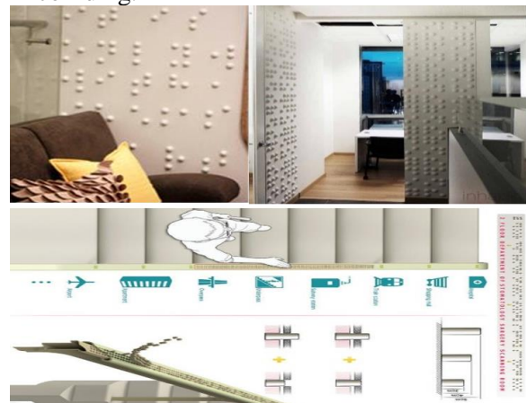
Fig (15) Hand support should be put on both sides of the walls at a height of 85 cm to 95 cm, and ideally in the cushions, with a diameter of 40mm to 50mm.
