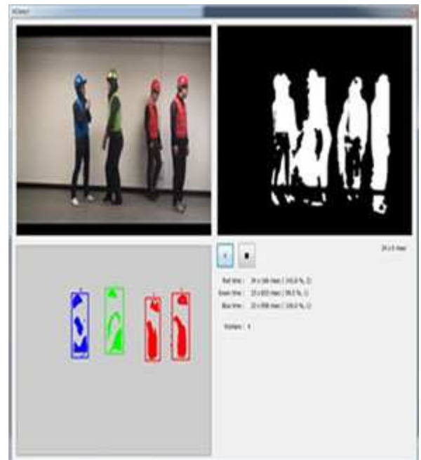
Fig. 7: Implemented system for counting man-hours of each construction worker group
