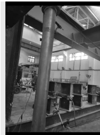
Figure (3) Specimen testing configuration of long column
