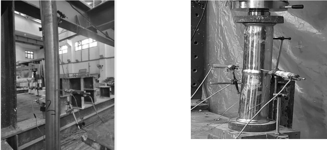
Figure (5): Experimental failure mode for column specimen C1400/12 and C500/12 Experimental results of load-axial shortening relationship for column specimens C1400/12 C1400/26 shown in Figure (6) and Figure (7).
