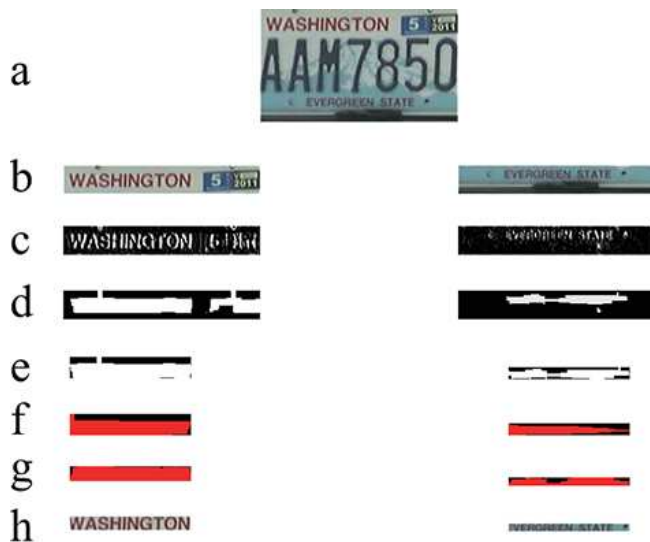
Fig. 9: The state name refinement procedure: (a) an original license plate, (b) the upper and lower region, (c) the Sobel and binarized results, (d) the morphology results, (e) the bounding box satisfying formula (9), (f) the horizontal projection, (g) the vertical projection, and (h) the refinement result.
