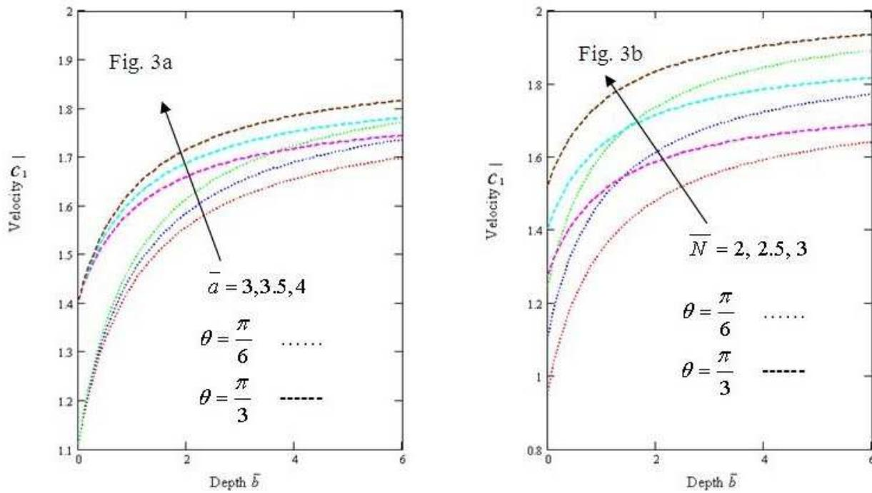
Fig. 3: Variation of velocity  $\overline{C_1}$  with respect to the depth with variation of (a)  $\overline{a}$  and (b)  $\overline{N}$ .
