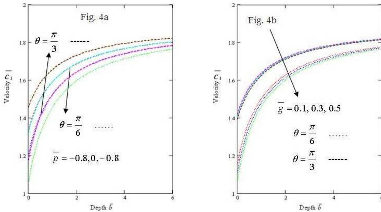
Fig. 4: Variation of velocity  $\overline{C_1}$  with respect to the depth with variation of (a)  $\overline{p}$  and (b)  $\overline{g}$ .
