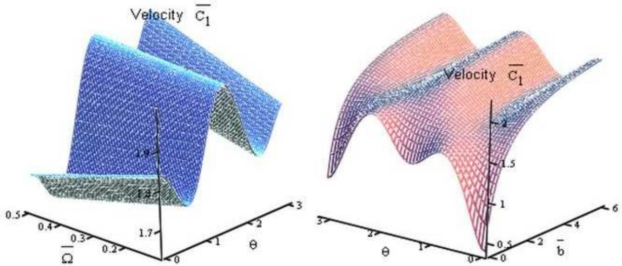
Fig. 12: Variation of velocity  $\bar{C}_1$  with respect to  $(\bar{\Omega}, \bar{\theta})$  and  $(\bar{h}, \bar{b})$ .
