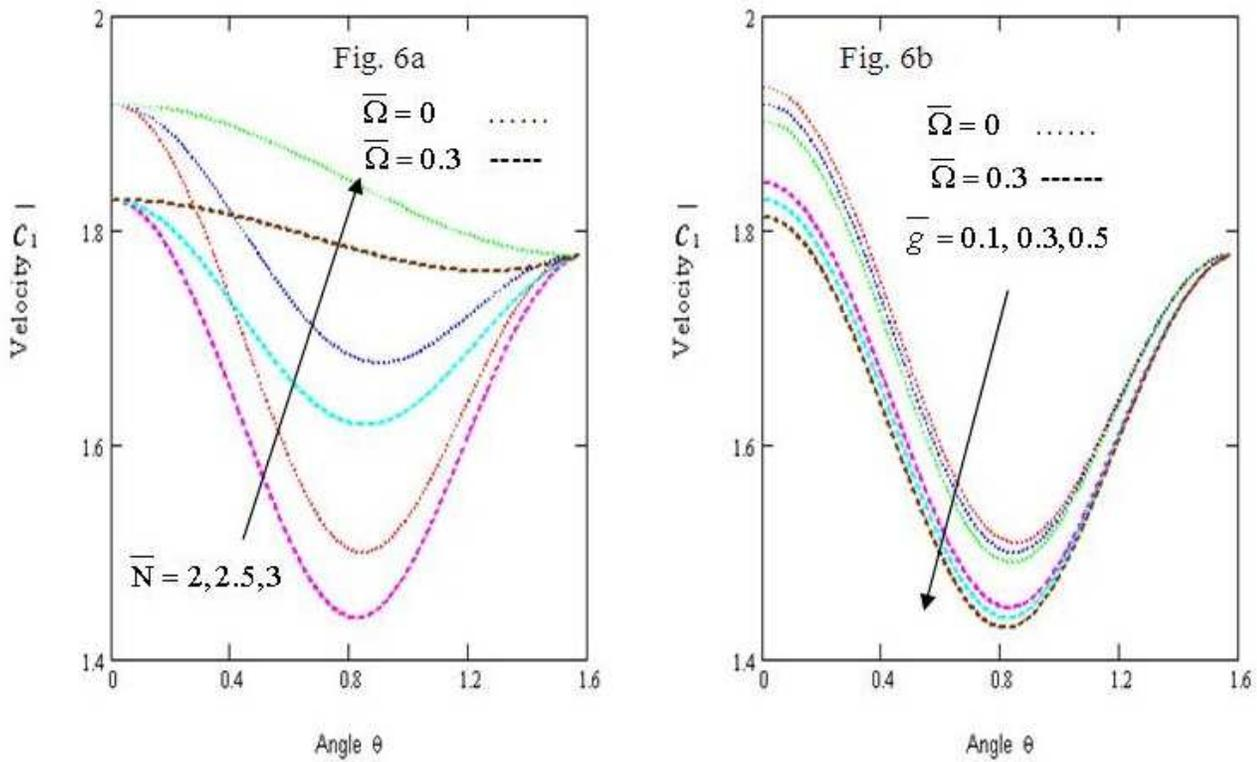
Fig. 6: Variation of velocity  $\bar{C}_1$  with respect to the depth with variation of (a)  $\bar{N}$  and (b)  $\bar{g}$ .
