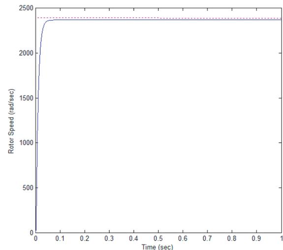
**Fig. 4:** Rotate speed simulation using  $\mathcal{H}_\infty$  fuzzy controller based on LMI with load change.
