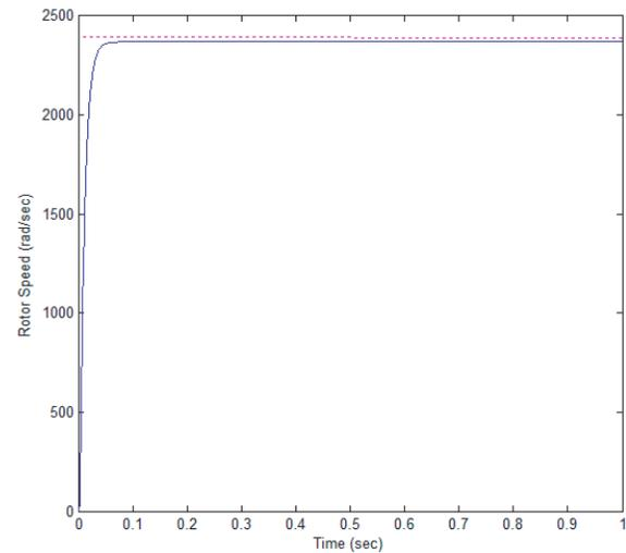
**Fig. 3:** Rotate speed simulation using  $\mathcal{H}_\infty$  fuzzy controller based on LMI with no load.
