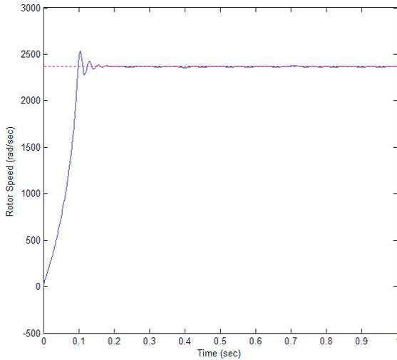
**Fig. 5:** Rotate speed simulation using PID controller with load change.
