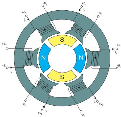
Fig. 1: Basic three-phase, 4 poles brushless motor.
