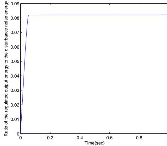
**Fig. 7:** The ratio of the regulated output energy to the disturbance noise energy:  $\left( \frac{\int_0^T z^T(t)z(t)dt}{\int_0^T w^T(t)w(t)dt} \right)$
