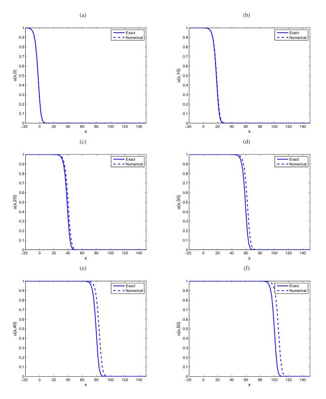
Fig. 2: Graphs of the exact (solid) and the approximate (dashed) solutions of (1). The exact solution is given by (30), and the approximations have been obtained through (7) at the times (a) t = 0, (b) t = 10, (c) t = 20, (d) t = 30, (e) t = 40 and (f) t = 50. The following computer parameters were used:  $\Omega = [-20, 150]$ ,  $\Delta x = 2$ ,  $\Delta t = 0.01$ , and  $\kappa = 1$ . Meanwhile, the initial profile was given by the exact solution at the time t = 0.
