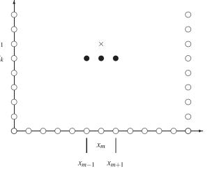
**Fig. 1:** Forward-difference stencil of the finite-difference method (7) at the time  $t_k$  around the node  $x_m$ . The black circles represent the known approximations to the exact solution at time  $t_k$ , and the cross denotes the unknown approximation at time  $t_{k+1}$ .
