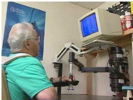
Figure. 1 Planar module of MIT-MANUS
