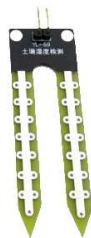
Fig. 1: The YL-69 sensor. It is used to read the soil moisture content around it.
