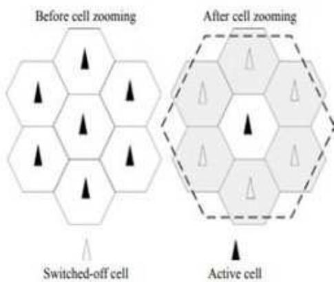
Fig. 2: Switch OFF BS before and after cell zooming
