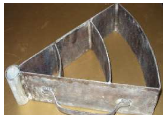
Fig. 3: Mould for preparing cylindrical sector elements
