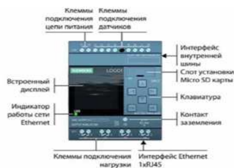
Figure 1: Layout of RC-2 and general view of PLC LOGO ! 230 RCE.
