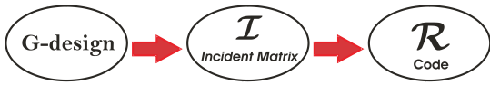
Fig. 5: A flow chart for the process of building codes from the graph design.
